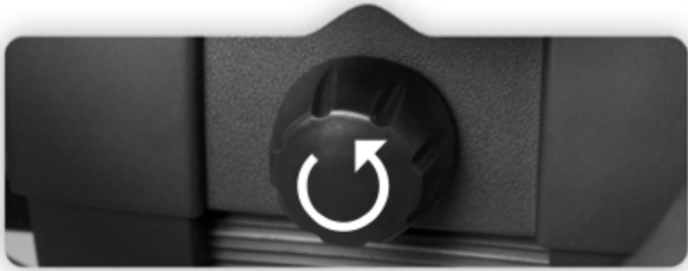
2. Pull out the table clamp while the wheel (rim) is facing the floor.
