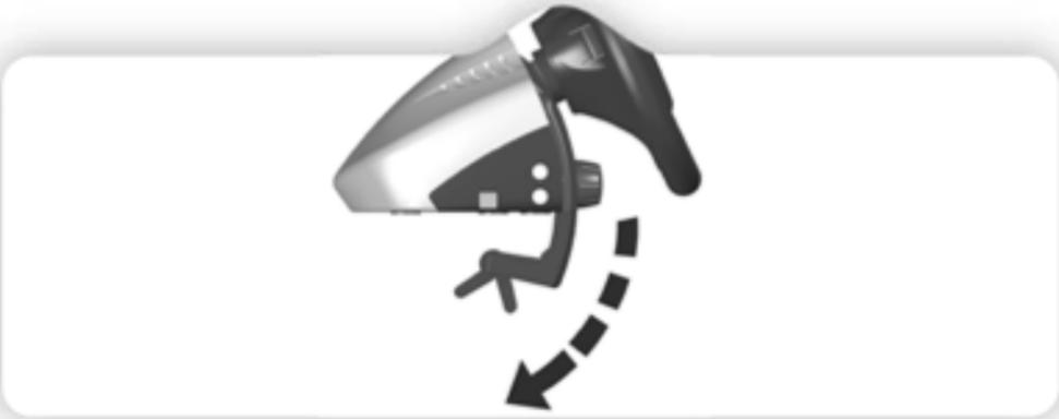
3. Mount the wheel to the table and then push in the table clamp as much as possible. Please note that the quick release clamps must be unfastened, and then tighten the table clamp screw.
